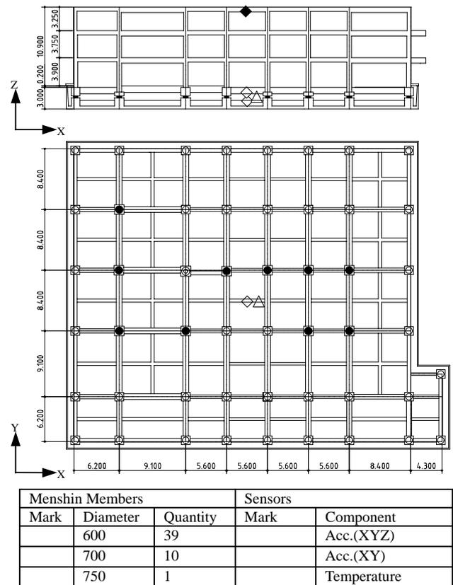
Fig.-1 Outline of Structure and Arrangement of Sensors
