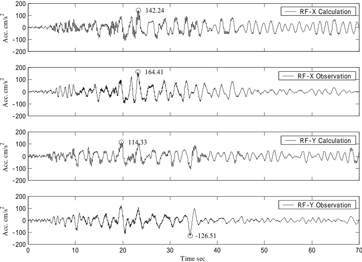
**Fig.-9 Comparison between Simulated and Observed Time History of Acceleration**
