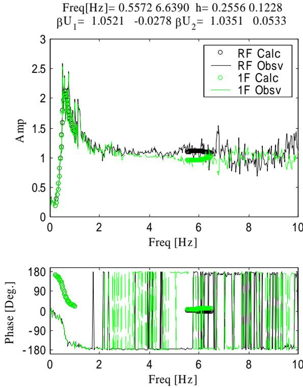
Fig.-7(a) Result of Curve Fit (Tokachi-oki)
