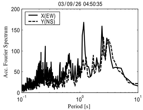
**Fig.-4(b) Fourier Spectrum of Tokachi-oki at the Base**
