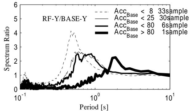
**Fig.-6 Transfer Function by Observation (RF/Base)**
