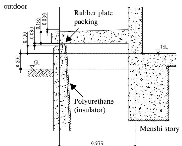
Fig.-3 Rubber Plate Packing
