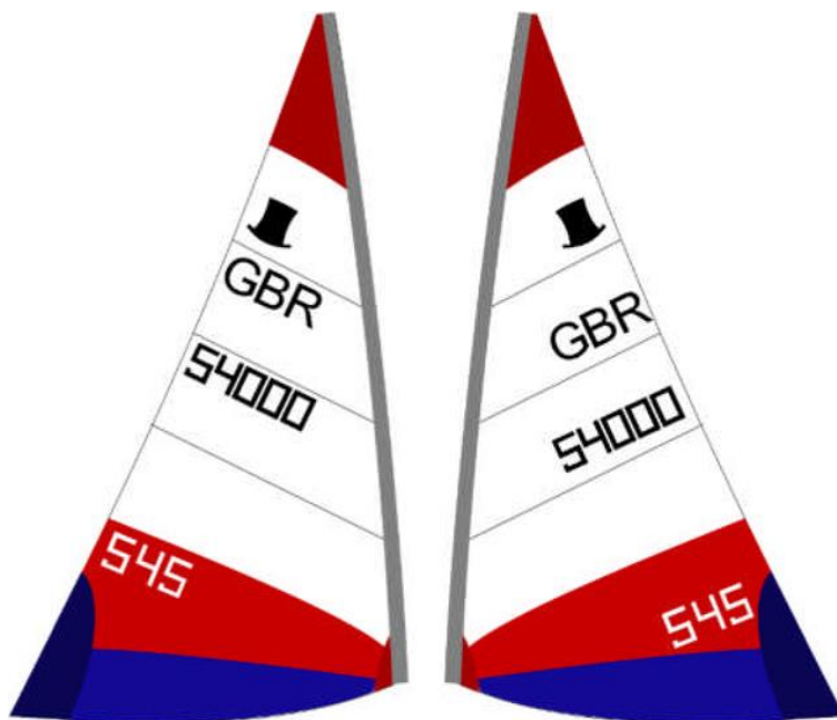
Figure 13 Sail starboard and port with the correct placing of National Letters, Sail Number and Event Number.
